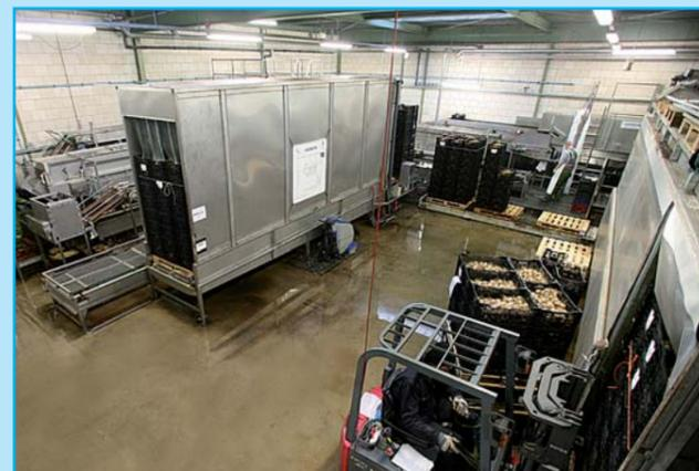
Of course, washing and cleaning is an important process for the further development of the flower bulbs. Here we are striving to the maximum to perform this work as perfect as possible. Therefore, our machinery chain is completely made of stainless steel, to avoid the transfer of the virus during the process. The level of our water reservoir is maintained by rain fall and has a capacity of over 1500 m<sup>3</sup>. The return water is perfectly clean for reuse.
